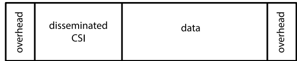
Fig. 1. Example fixed-length packet showing overhead, data, and CSI dissemination. The CSI dissemination consists of M \in \{1, \dots, N-1\} channel estimates where the length of each channel estimate is one word. The data and overhead consist of D words. The total packet length is P = M + D words.
