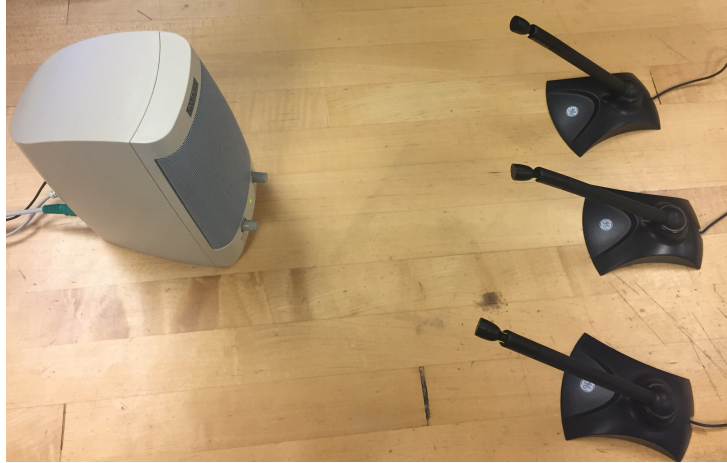
Figure 2: Experimental Setup of Multiuser Acoustic Transmitter and Three Receivers
